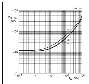
Transistor TR1;  $I_C/I_B = 20$ .
