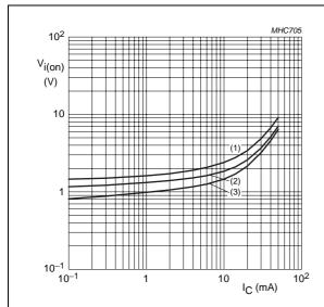
Transistor TR2;  $V_{CE} = 0.3 \text{ V}.$
