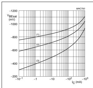
Transistor TR1;  $I_C/I_B = 20$ .
