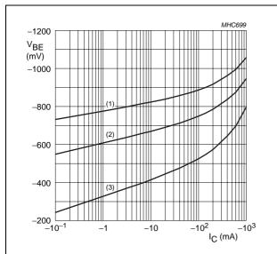
Transistor TR1;  $V_{CE} = -2 V$ .
