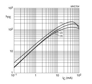
Transistor TR2;  $V_{CE} = 5 \text{ V}$ .
