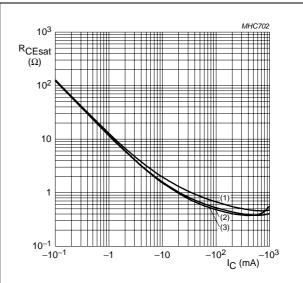
Transistor TR1;  $I_C/I_B = 20$ .
