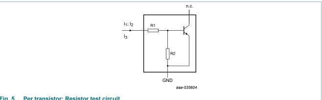
Fig. 5. Per transistor: Resistor test circuit
