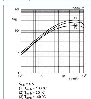
DC current gain as a function of collector Fig. 1. current; typical values
