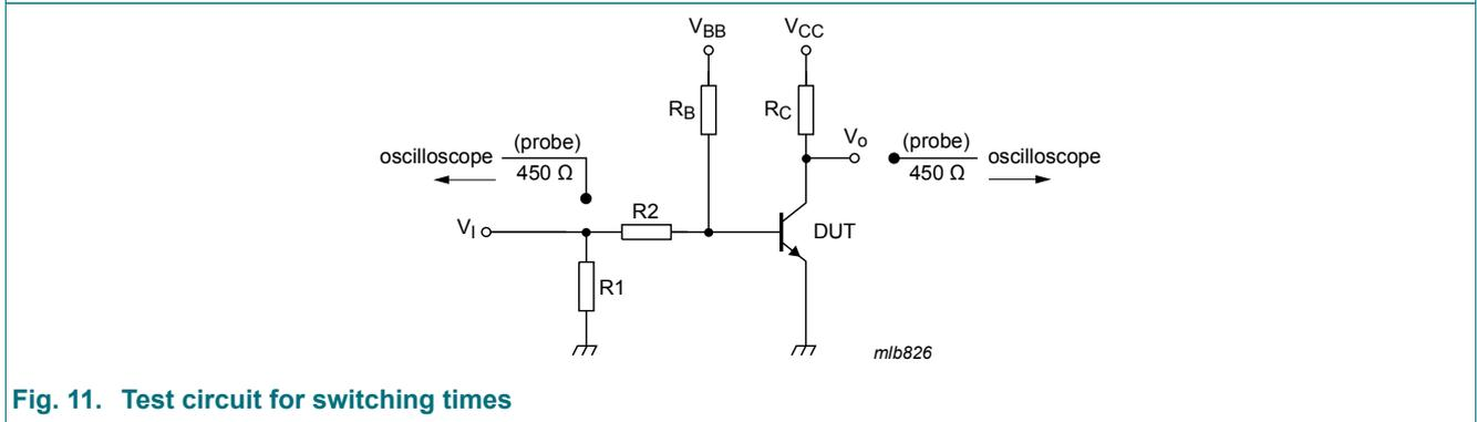
Fig. 11. Test circuit for switching times
