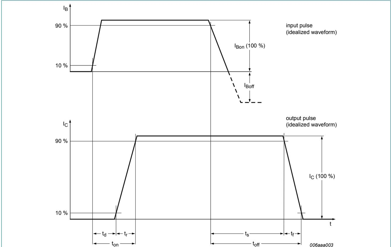
Fig. 10. Transistor switching time definition
