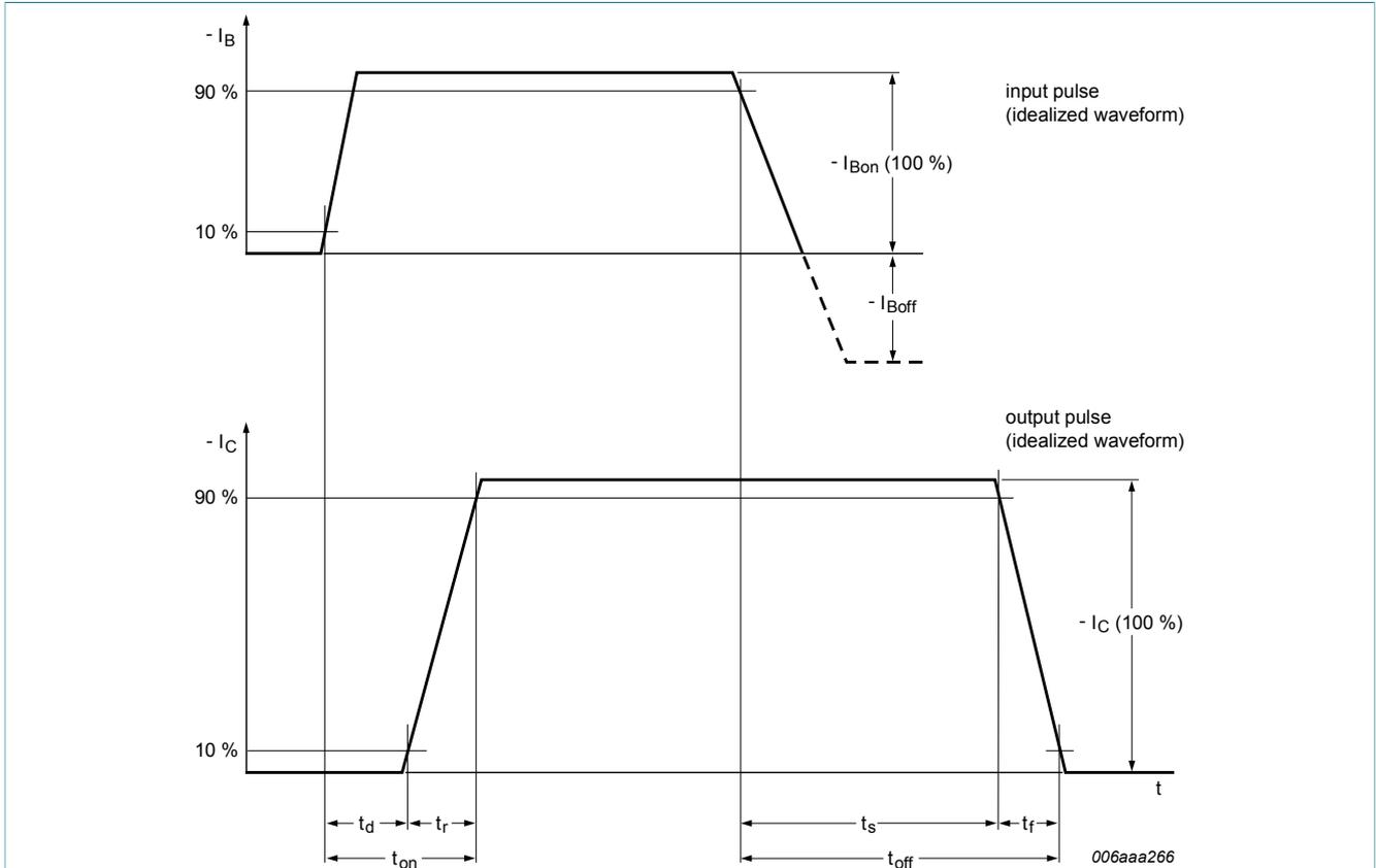
Fig. 10. BISS transistor switching time definition
