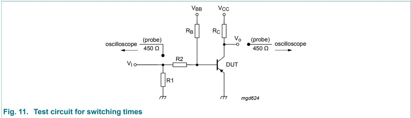
Fig. 11. Test circuit for switching times
