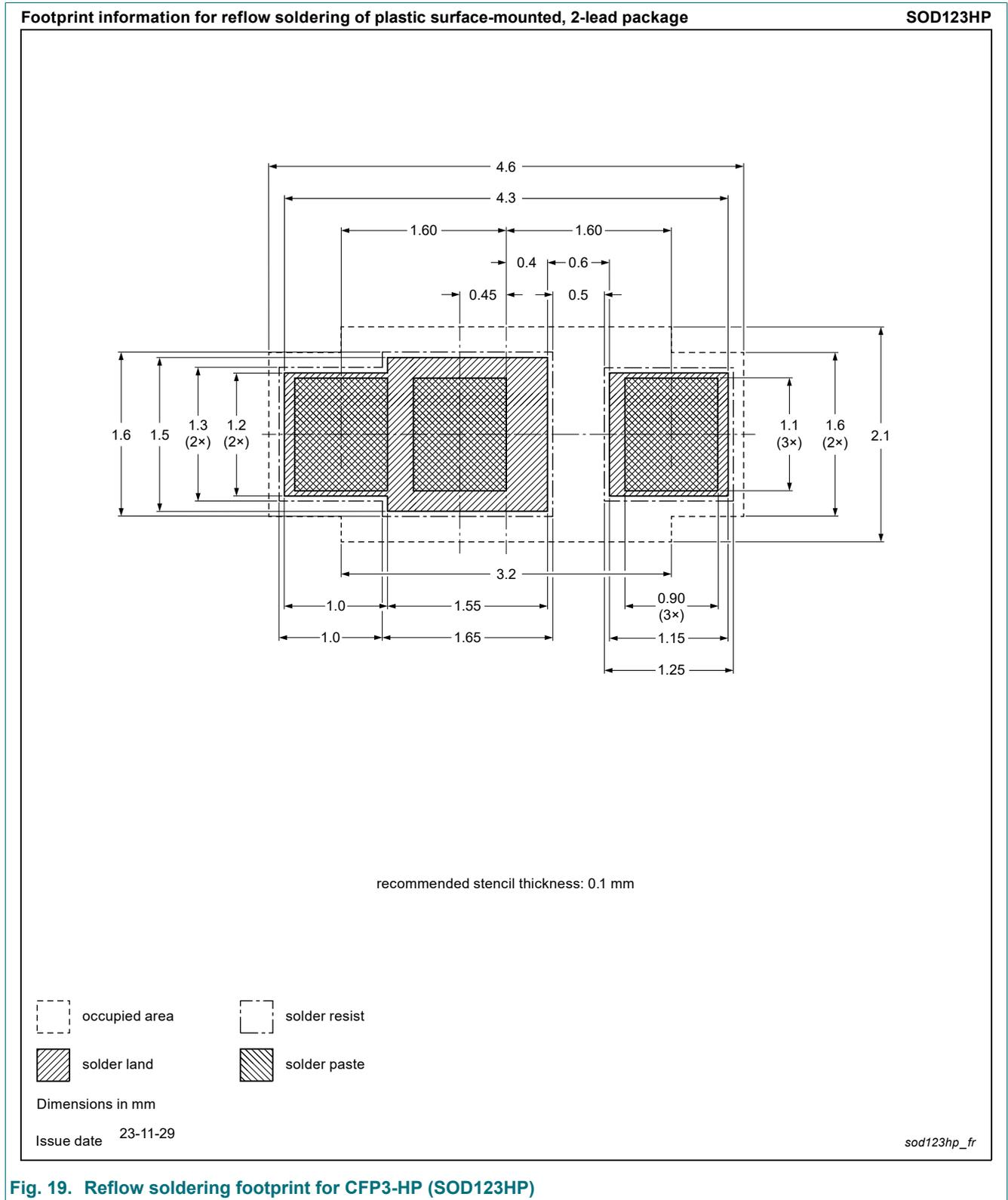
Fig. 19. Reflow soldering footprint for CFP3-HP (SOD123HP)
