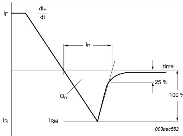
Fig. 15. Reverse recovery definition; ramp recovery
