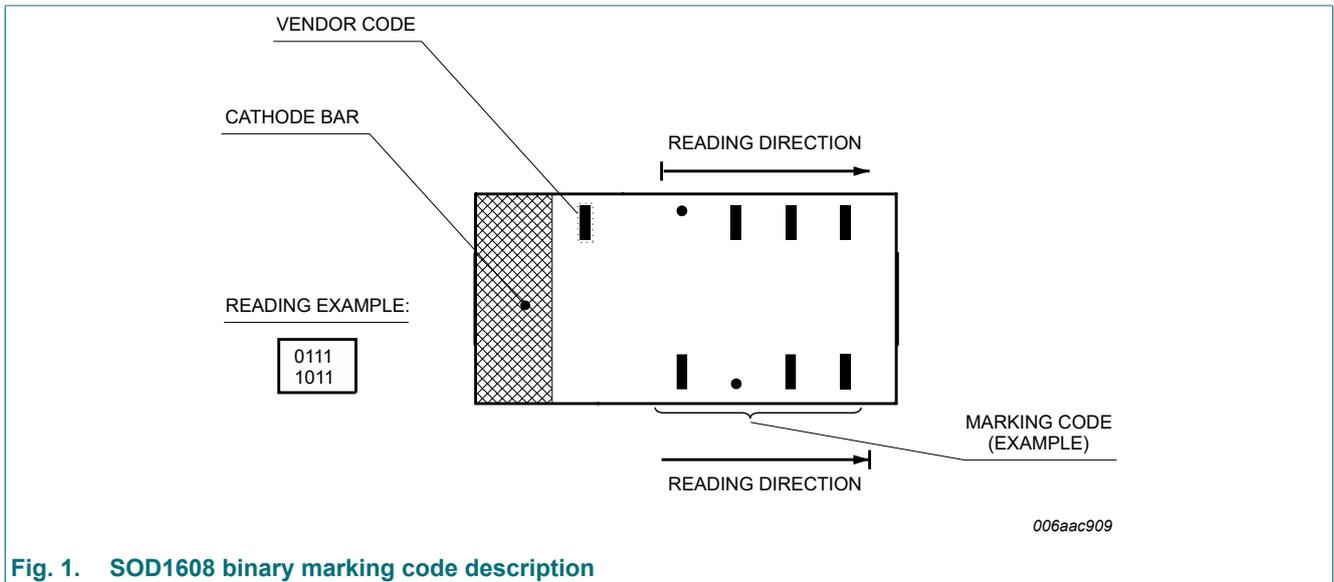
Fig. 1. SOD1608 binary marking code description
