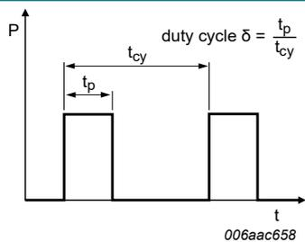
Fig. 16. Duty cycle definition
