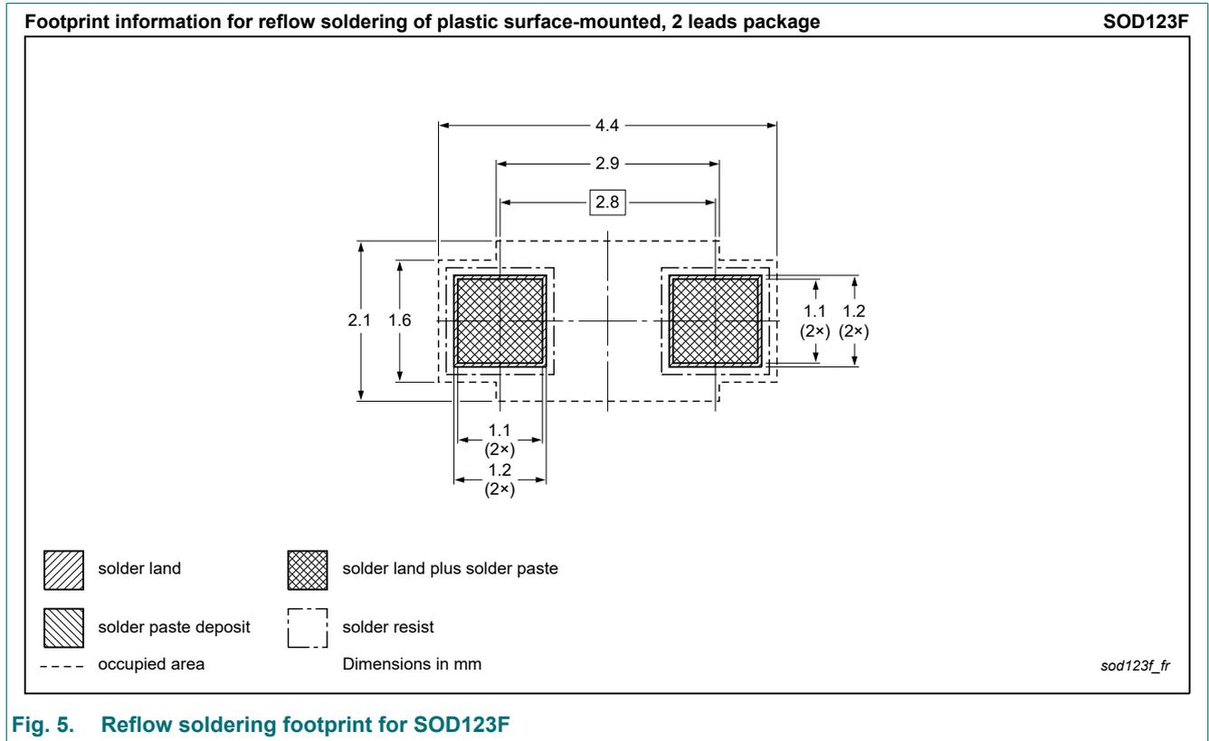
Fig. 5. Reflow soldering footprint for SOD123F
