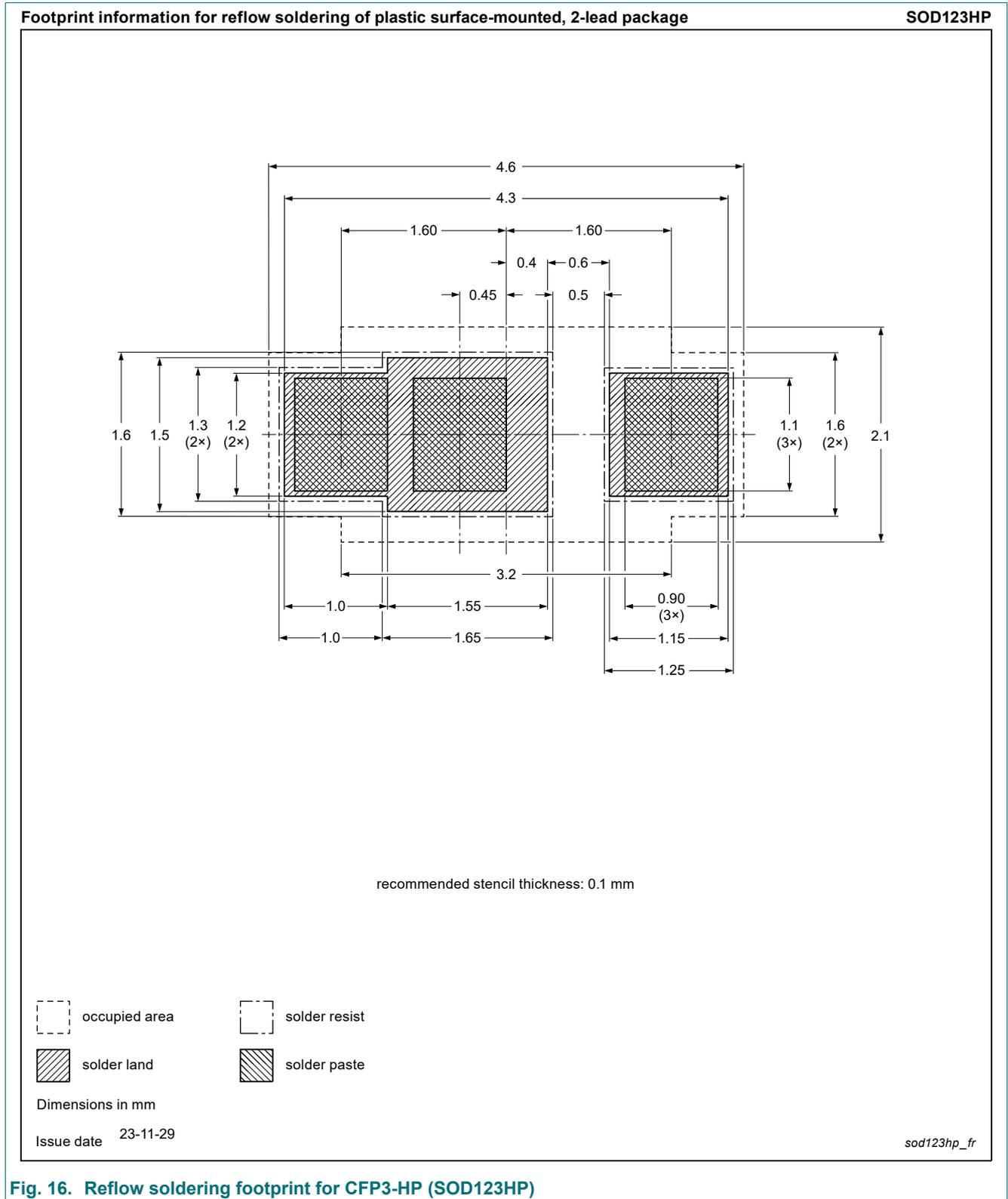
Fig. 16. Reflow soldering footprint for CFP3-HP (SOD123HP)
