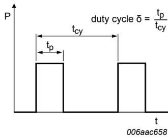
Fig. 14. Duty cycle definition
