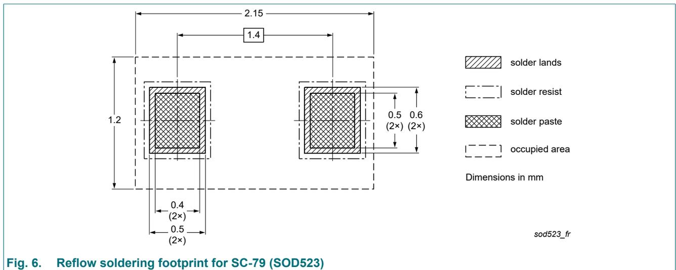
Fig. 6. Reflow soldering footprint for SC-79 (SOD523)
