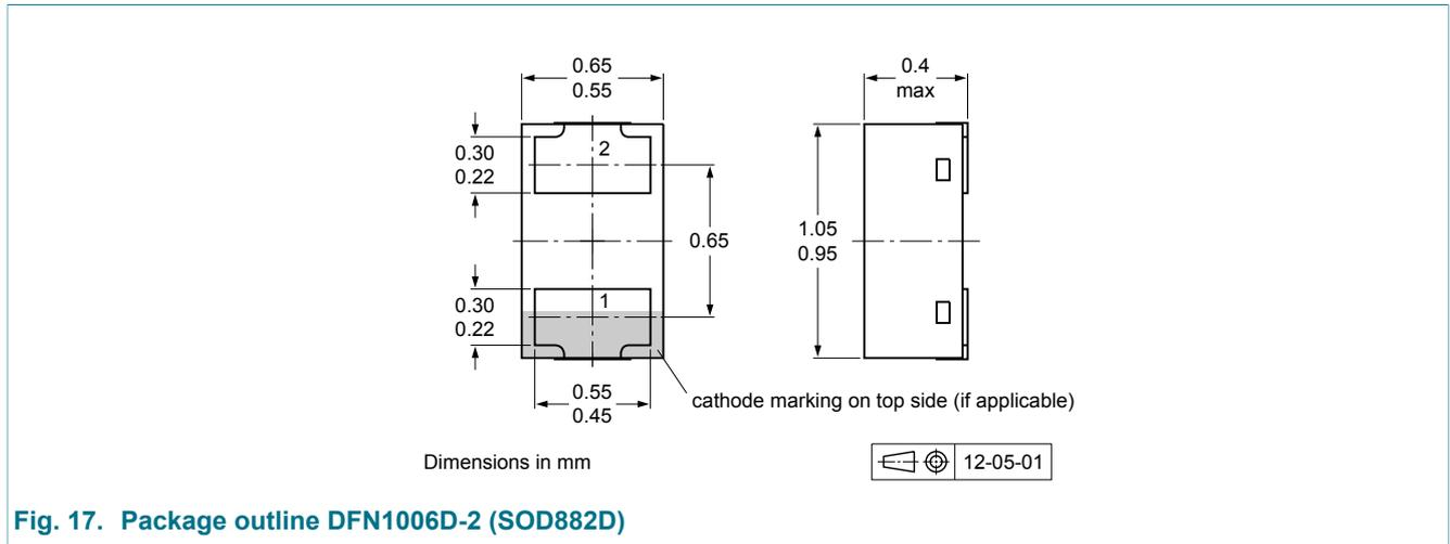
Fig. 17. Package outline DFN1006D-2 (SOD882D)
