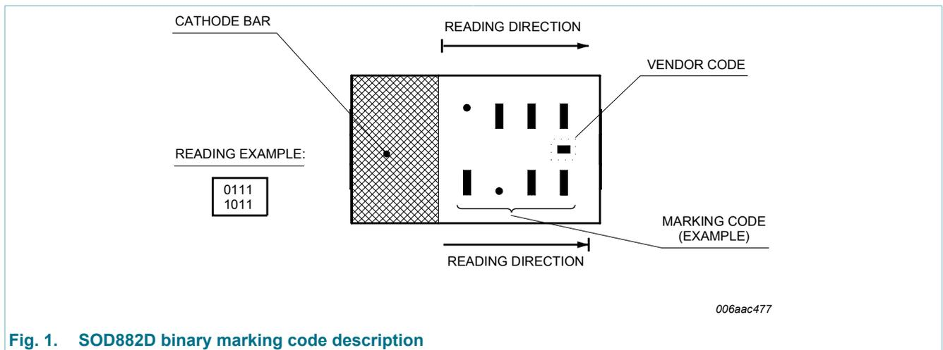
Fig. 1. SOD882D binary marking code description
