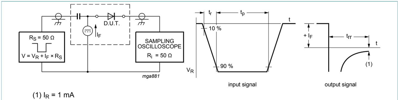
Fig. 15. Reverse recovery time: test circuit and waveforms
