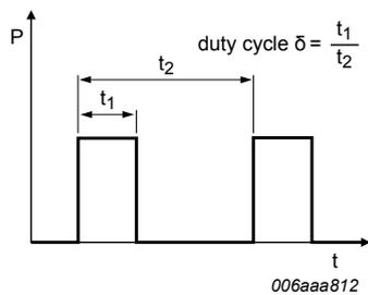
Fig. 14. Duty cycle definition
