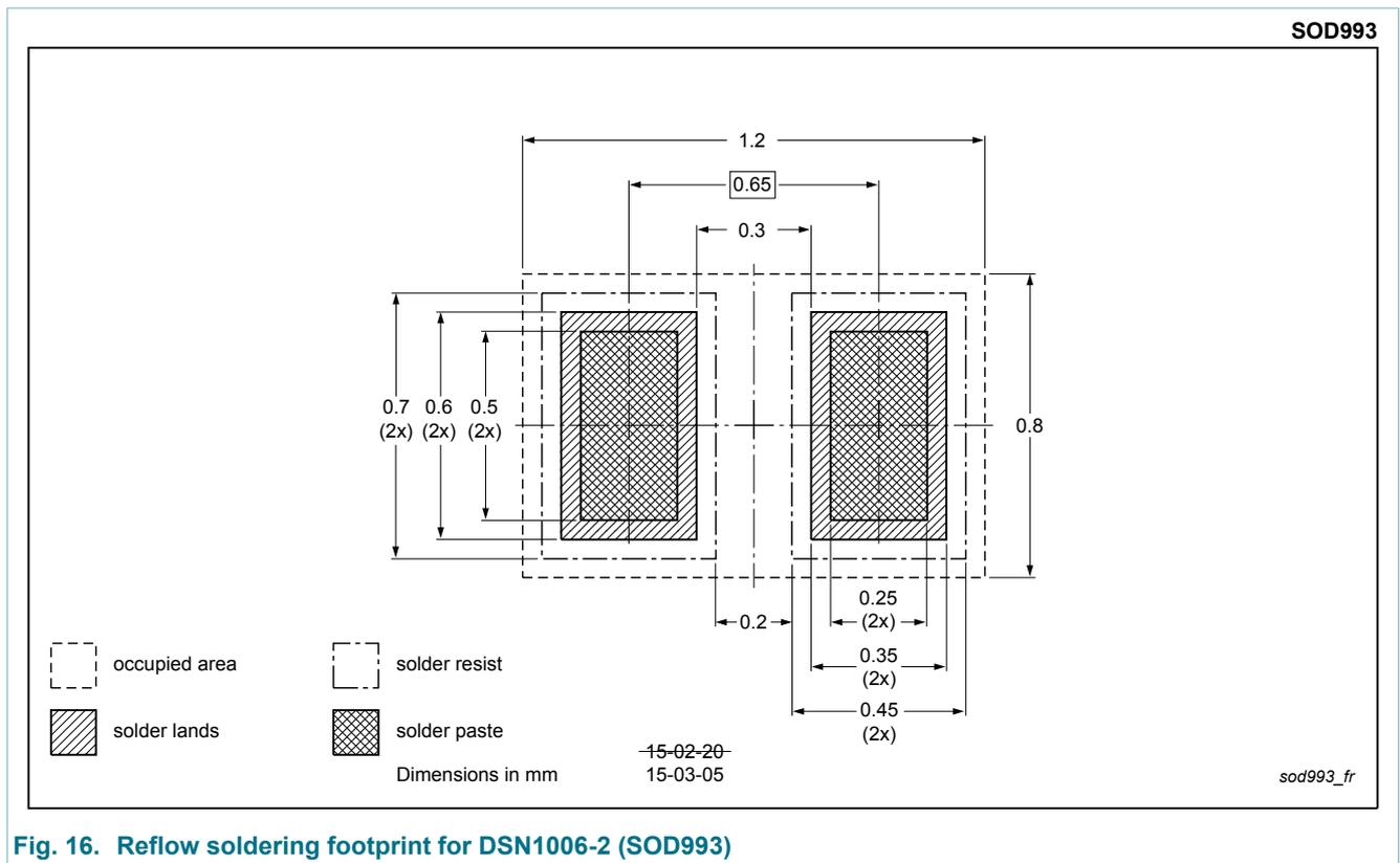
Fig. 16. Reflow soldering footprint for DSN1006-2 (SOD993)
