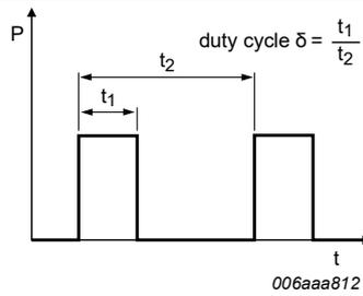
Fig. 6. Duty cycle definition
