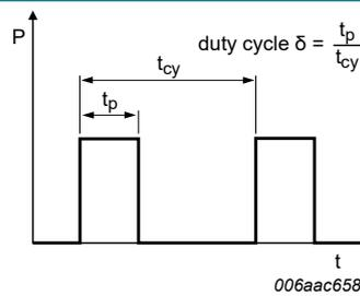
Fig. 17. Duty cycle definition
