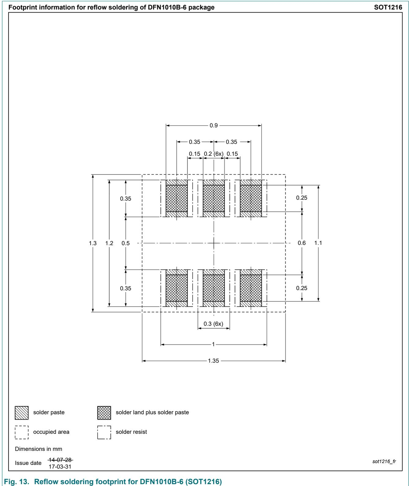
Fig. 13. Reflow soldering footprint for DFN1010B-6 (SOT1216)
