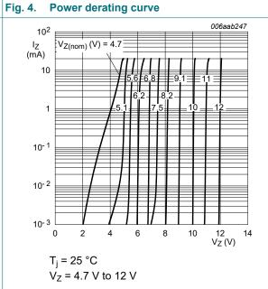
Fig. 6. Working current as a function of working voltage; typical values
