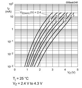
Fig. 5. Working current as a function of working voltage; typical values
