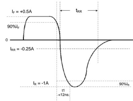
Figure 7 Reverse Recovery Time Characteristics and Test Circuit
