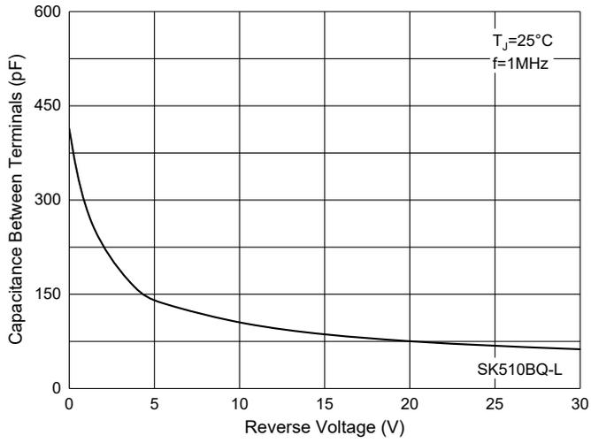
Fig. 8 - Capacitance Characteristics
