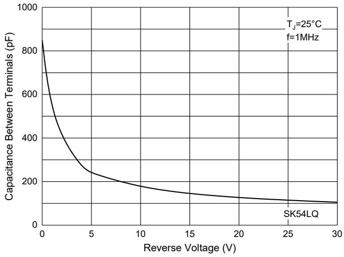
Fig. 8 - Capacitance Characteristics
