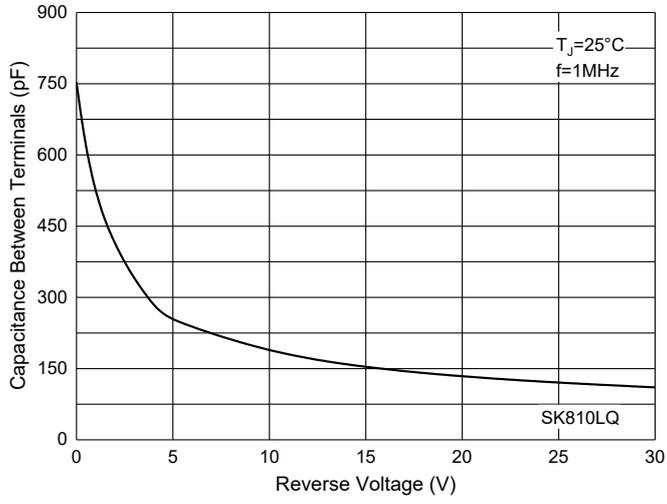
Fig. 8 - Capacitance Characteristics
