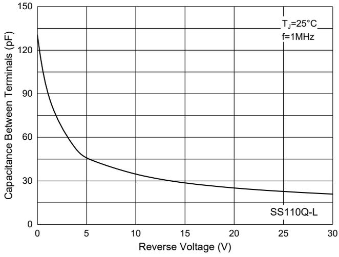
Fig. 8 - Capacitance Characteristics
