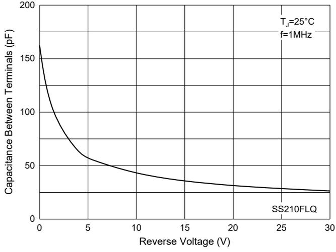
Fig. 8 - Capacitance Characteristics
