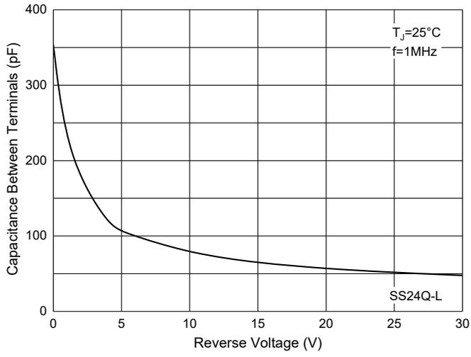
Fig. 8 - Capacitance Characteristics
