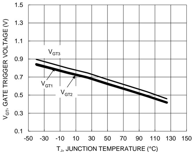
Figure 5. Typical Gate Trigger Voltage vs. Junction Temperature
