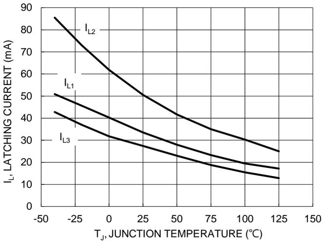
Figure 9. Typical Latching Current vs. Junction Temperature
