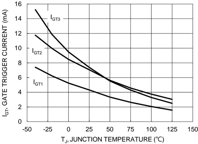
Figure 1. Typical Gate Trigger Current vs. Junction Temperature
