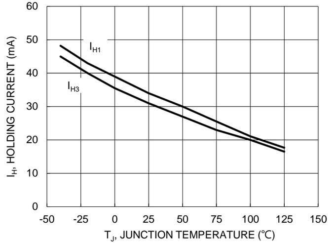
Figure 8. Typical Holding Current vs. Junction Temperature
