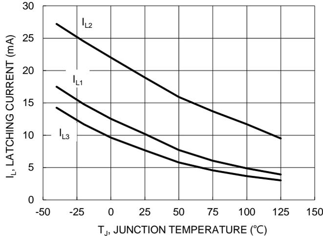
Figure 3. Typical Latching Current vs. Junction Temperature
