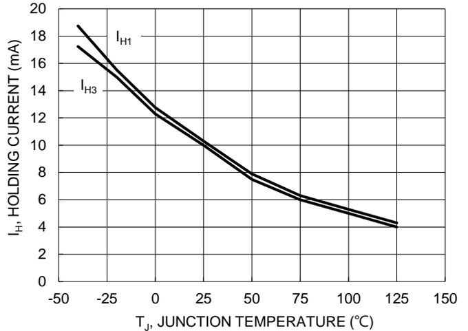
Figure 2. Typical Holding Current vs. Junction Temperature
