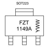
FZT 1149A = Product Type Marking Code YWW = Date Code Marking Y or  $\overline{Y}$  = Last Digit of Year (ex: 5= 2015) WW or  $\overline{W}W$  = Week Code (01~53)
