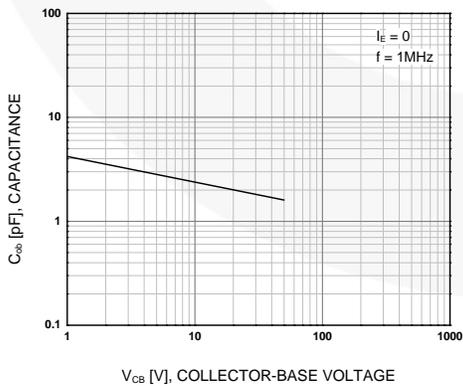
Figure 5. Output Capacitance
