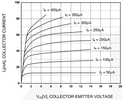
Figure 1. Static Characteristic
