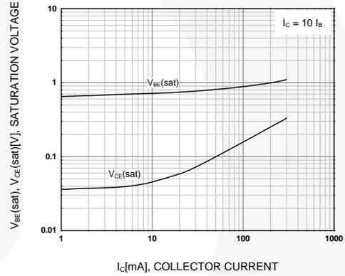
Figure 4. Base-Emitter Saturation Voltage and Collector-Emitter Saturation Voltage
