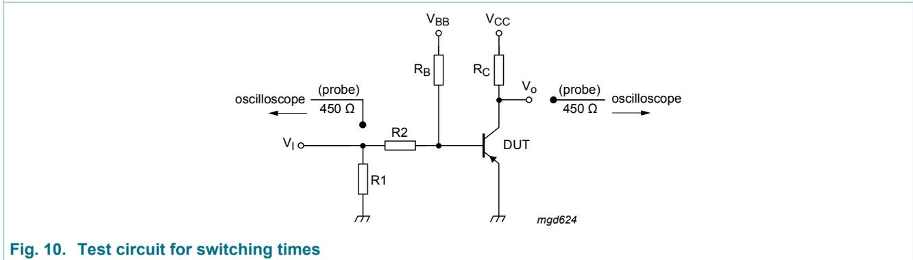
Fig. 10. Test circuit for switching times
