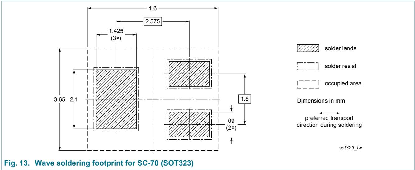
Fig. 13. Wave soldering footprint for SC-70 (SOT323)
