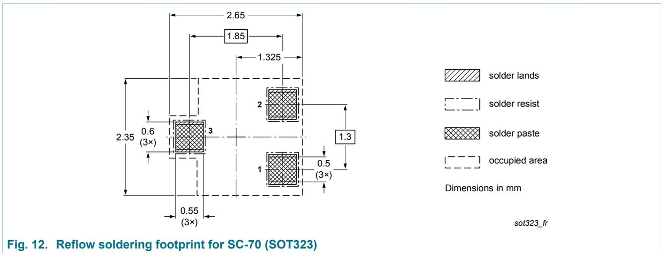
Fig. 12. Reflow soldering footprint for SC-70 (SOT323)
