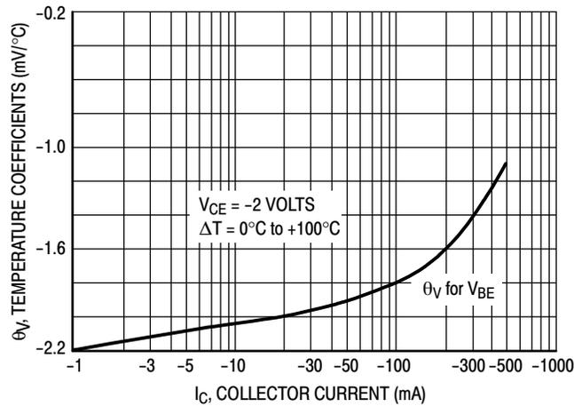
Figure 5. Temperature Coefficients
