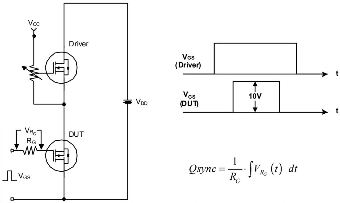
Figure 18. Total Gate Charge  $Q_{sync}$ . Test Circuit & Waveforms
