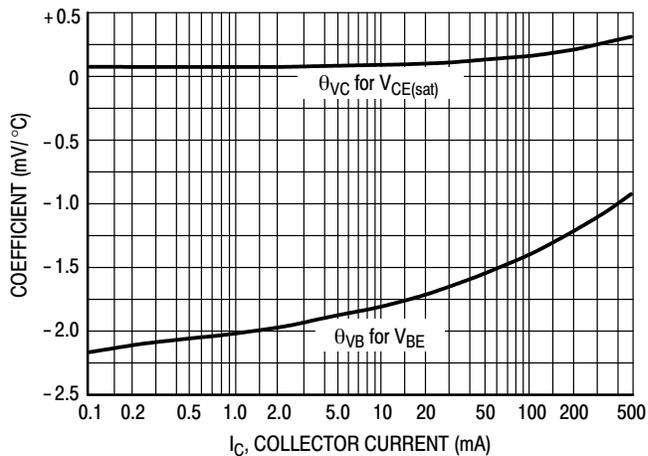
Figure 16. Temperature Coefficients
