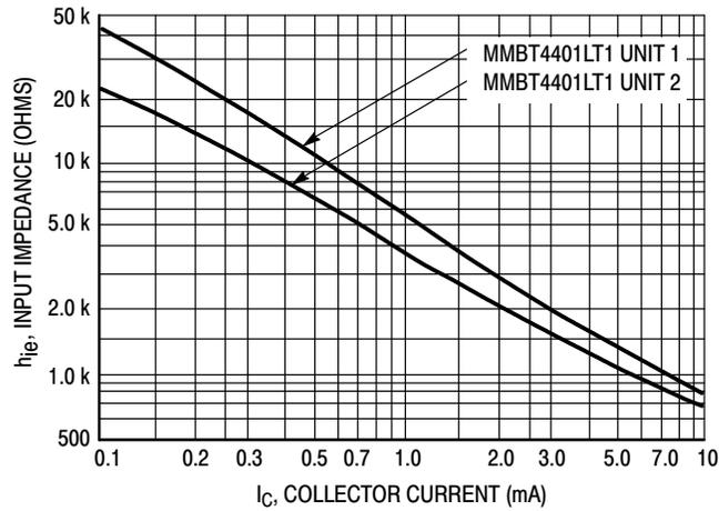
Figure 10. Input Impedance
