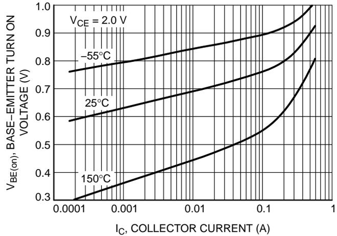
**Figure 18. Base-Emitter Turn On Voltage vs. Collector Current**
