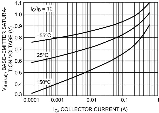
**Figure 17. Base-Emitter Saturation Voltage vs. Collector Current**
