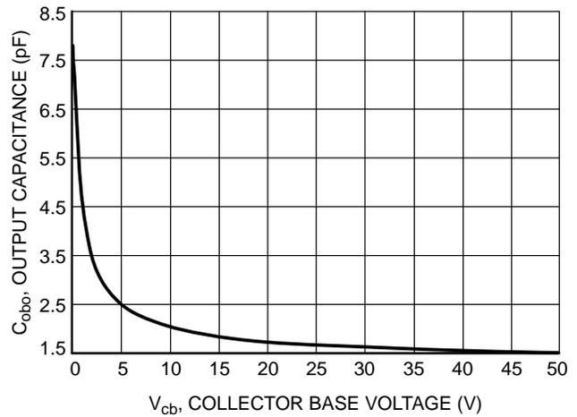
**Figure 20. Output Capacitance vs. Collector Base Voltage**
