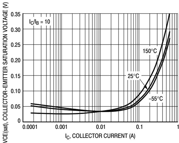
Figure 15. Collector-Emitter Saturation Voltage vs. Collector Current
