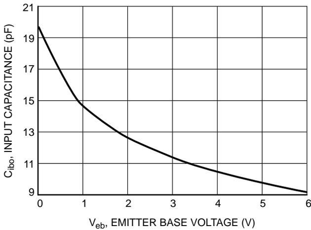
**Figure 19. Input Capacitance vs. Emitter Base Voltage**
