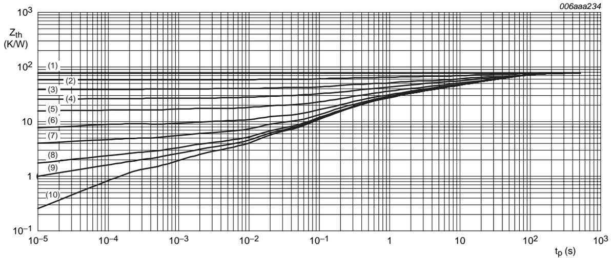
Mounted on FR4 printed-circuit board; mounting pad for collector 6 cm<sup>2</sup>.
