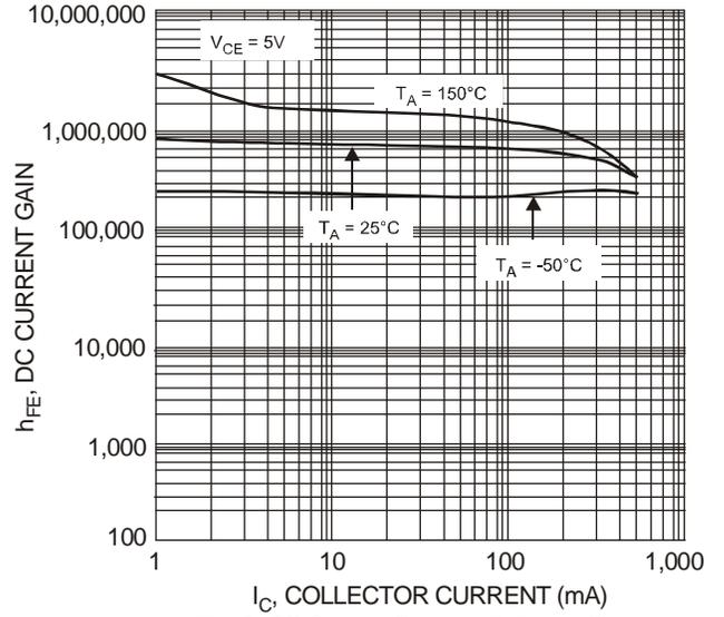
Fig. 3, DC Current Gain vs. Collector Current
