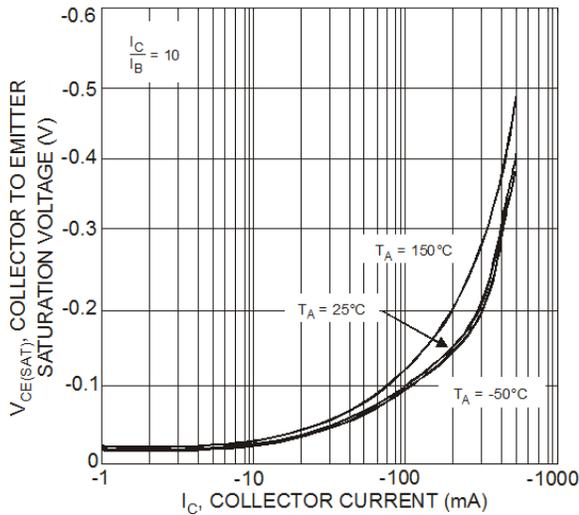
Fig. 4 Collector-Emitter Saturation Voltage vs. Collector Current
