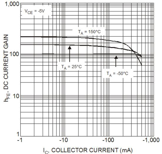
Fig. 5 DC Current Gain vs. Collector Current
