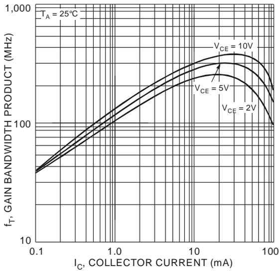
Fig. 4, Gain Bandwidth Product vs Collector Current
