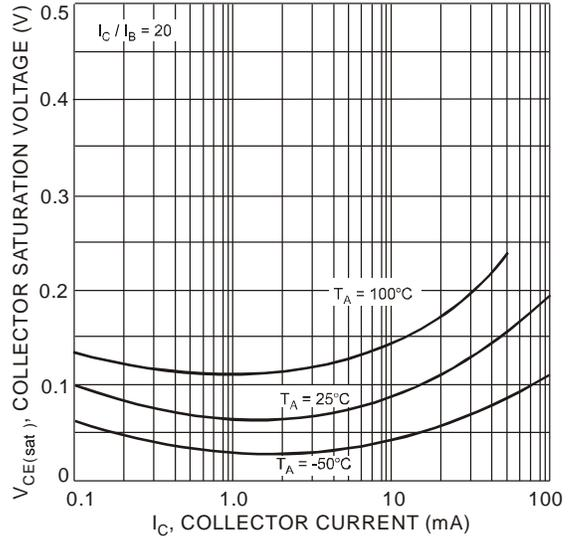
Fig. 3, Collector Saturation Voltage vs Collector Current
