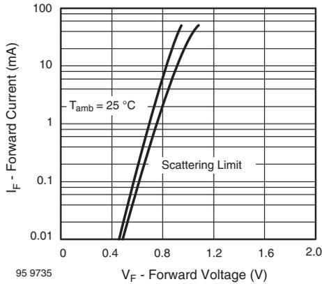
Fig. 1 - Forward Current vs. Forward Voltage
