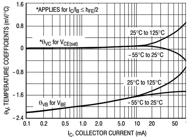
Figure 12. Temperature Coefficients
