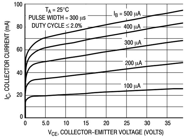
Figure 10. Collector Characteristics
