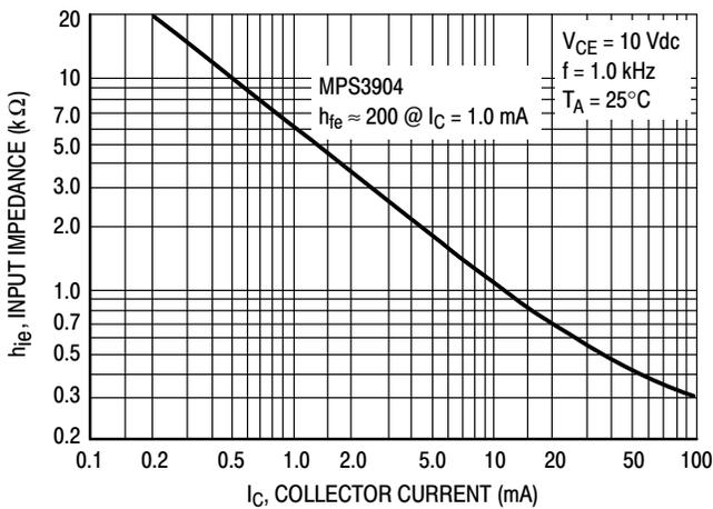
Figure 17. Input Impedance
