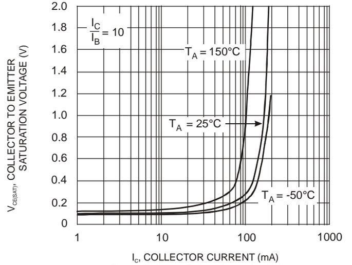
Fig. 2, Collector Emitter Saturation Voltage vs. Collector Current
