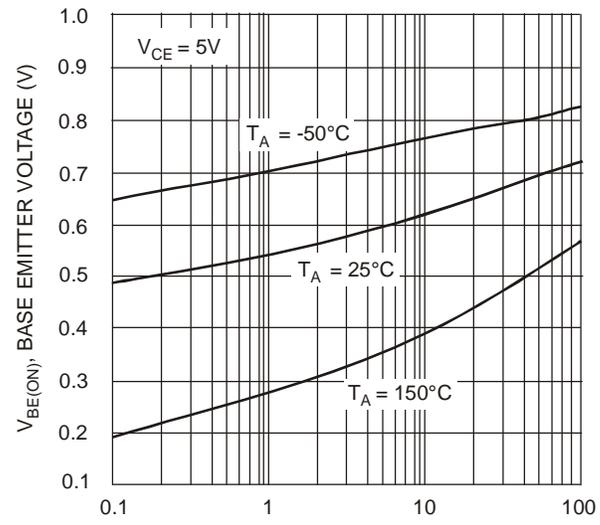
Fig. 4, Base Emitter Voltage vs Collector Current
