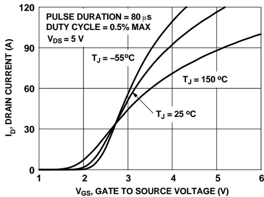
Figure 5. Transfer Characteristics
