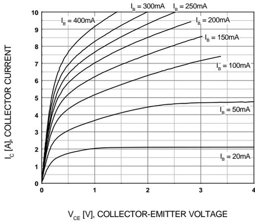
**Figure 1. Static Characteristic**
