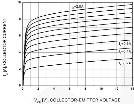
Figure 4. Static Characteristic
