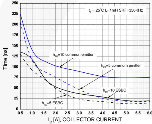
**Figure 12. Inductive Load Collector Current Fall-time ( $t_r$ )**
