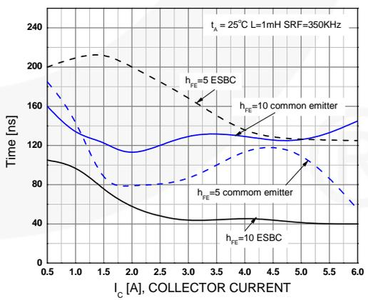
**Figure 15. Inductive Load Collector Voltage Rise-time ( $t_r$ )**
