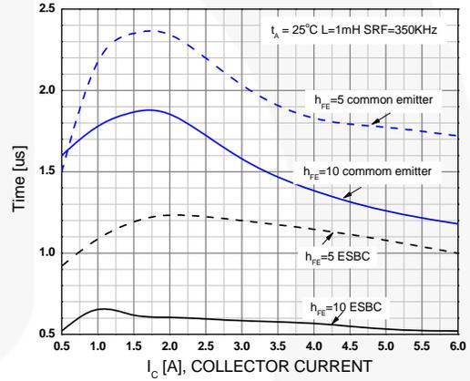
**Figure 13. Inductive Load Collector Current Storage time ( $t_{stg}$ )**
