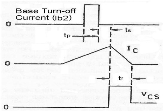
Figure 28. Storage Time - Common Emitter
