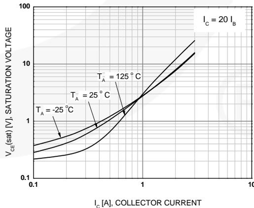
Figure 9. Collector-Emitter Saturation Voltage
