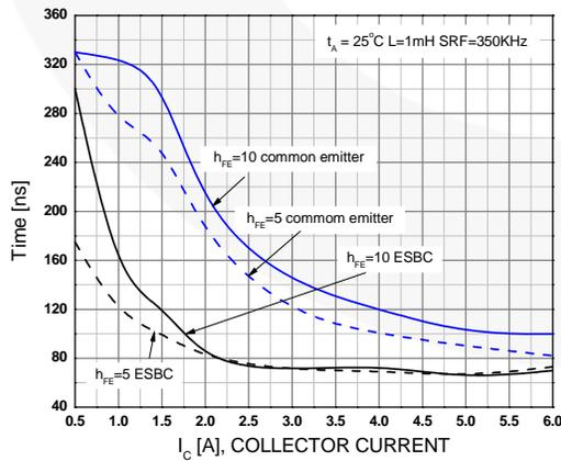
**Figure 14. Inductive Load Collector Voltage Fall-time ( $t_r$ )**
