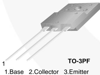
Figure 1. Pin Configuration
