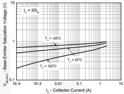
**Figure 8. Base-Emitter Saturation Voltage vs. Collector Current**
