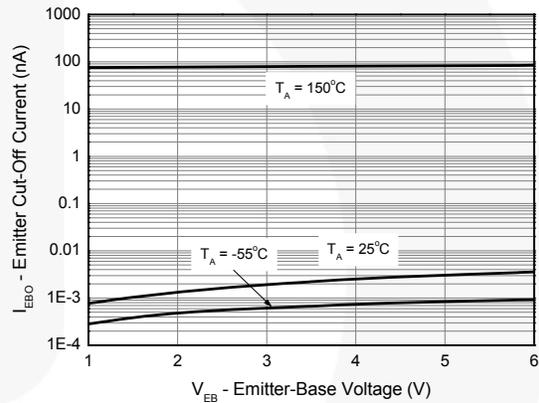
**Figure 10. Emitter Cut-Off Current vs. Emitter-Base Voltage**
