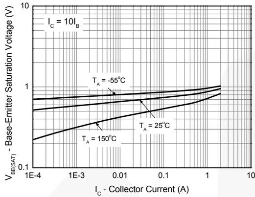
**Figure 7. Base-Emitter Saturation Voltage vs. Collector Current**
