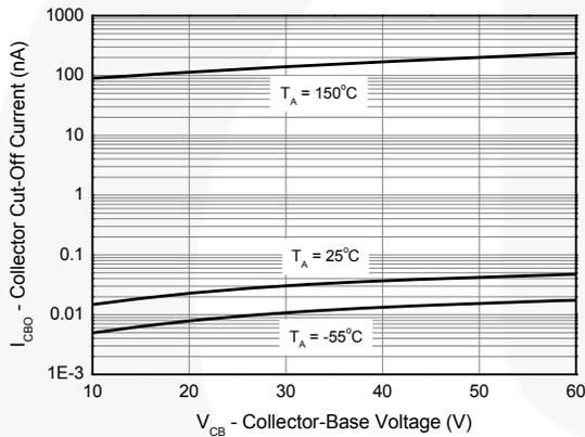
**Figure 9. Collector Cut-Off Current vs. Collector-Base Voltage**
