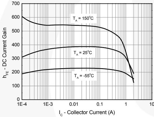
Figure 3. DC Current Gain vs. Collector Current
