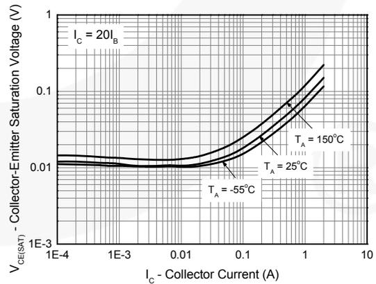
Figure 6. Collector-Emmitter Saturation Voltage vs. Collector Current
