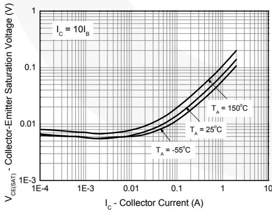
Figure 5. Collector-Emmitter Saturation Voltage vs. Collector Current
