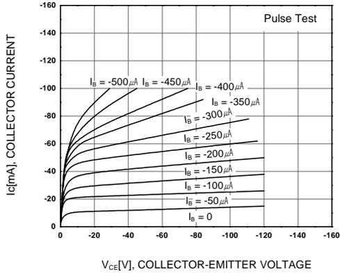
Figure 1. Static Characteristic
