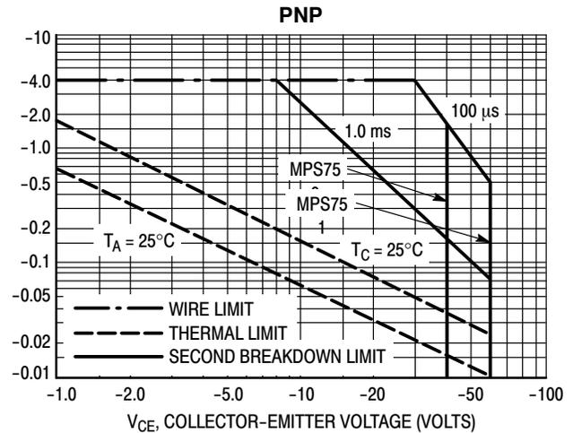
Figure 8. MPS750, MPS751 SOA, Safe Operating Area
