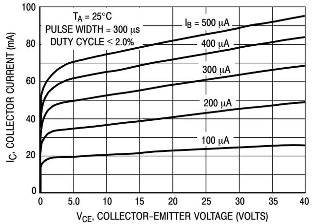
Figure 10. Collector Characteristics
