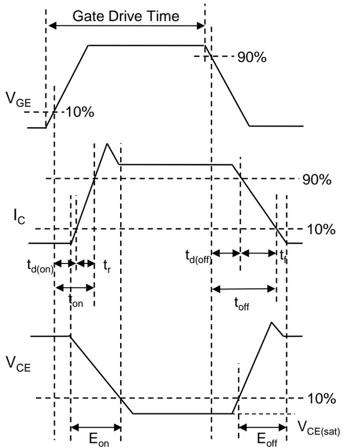
Fig.19 Inductive Load Waveform
