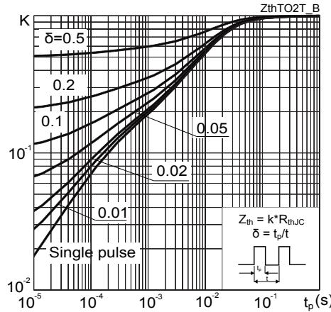
**Figure 28. Normalized transient thermal impedance for diode**
