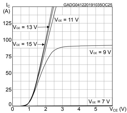
**Figure 6.** Typical output characteristics ( $T_J = 175 \text{ }^\circ\text{C}$ )
