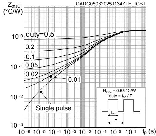
**Figure 27. TO-247 long leads normalized transient thermal impedance for IGBT**
