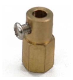
A coupling kit that can be used to connect the motor to the wheel, secure the motor shaft through the top wire on the coupling, and secure the coupling to the appropriate size wheel. The coupling is an 8 mm hex coupling with an inner diameter of 4 mm. Suitable for 6514A free wheel and 65 mm Mecanum and JGA25 motor
