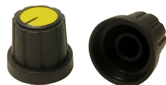
CP3505 - C18 KNOB WITH YELLOW CAP, 6mm SPLINE SHAFT WITH MARKER LINE. NOTE: CAP CANNOT BE REMOVED.
