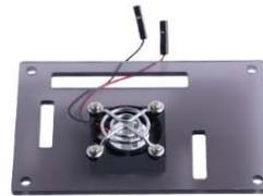
8. Connect the cables of cooling fan to GPIO headers!
