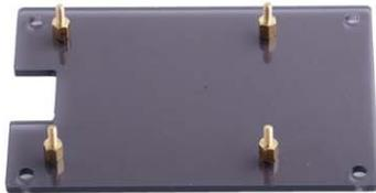
4. Put the Raspberry Pi Board on the acrylic panel as the picture shows and screw 4 nuts !
