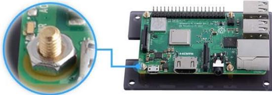
5. Pick out 4 big header screws and 4 long standoffs! Install 4 pieces of big header screws through the bottom panel and screw 4 long standoffs!
