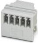
Header, nominal current: 8 A, rated voltage (III/2): 160 V, number of positions: 5, pitch: 3.5 mm, color: light gray, contact surface: Tin, mounting: Soldering, Article with lateral pin exit
