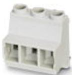
PCB terminal block, nominal current: 24 A, nom. voltage: 630 V, pitch: 7.5 mm, number of positions: 3, connection method: Screw connection with tension sleeve, mounting: Wave soldering, color: light gray. Article with lateral pin exit
