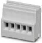
PCB terminal block, nominal current: 8 A, nom. voltage: 160 V, pitch: 3.5 mm, number of positions: 5, connection method: Screw connection with tension sleeve, mounting: Wave soldering, conductor/PCB connection direction: 0 °, color: light gray. Article with lateral pin exit
