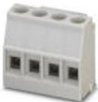
PCB terminal block, nominal current: 24 A, nom. voltage: 400 V, pitch: 5 mm, number of positions: 4, connection method: Screw connection with tension sleeve, mounting: Wave soldering, conductor/PCB connection direction: 0 °, color: light gray. Article with lateral pin exit
