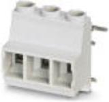
PCB terminal block, nominal current: 24 A, nom. voltage: 630 V, pitch: 7.5 mm, number of positions: 3, connection method: Screw connection with tension sleeve, mounting: Wave soldering, color: light gray. Article with lateral pin exit
