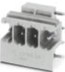
Header, nominal current: 16 A, rated voltage (III/2): 320 V, number of positions: 4, pitch: 5 mm, color: light gray, contact surface: Tin, mounting: Soldering
