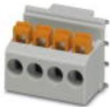
PCB terminal block, nominal current: 22 A, nom. voltage: 250 V, pitch: 5 mm, number of positions: 4, connection method: Push-in spring connection, mounting: Wave soldering, conductor/PCB connection direction: 0 °, color: light gray. Article with lateral pin exit
