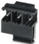
Header, nominal current: 16 A, rated voltage (III/2): 630 V, number of positions: 3, pitch: 7.25 mm, mounting: SMD/THT/THR
